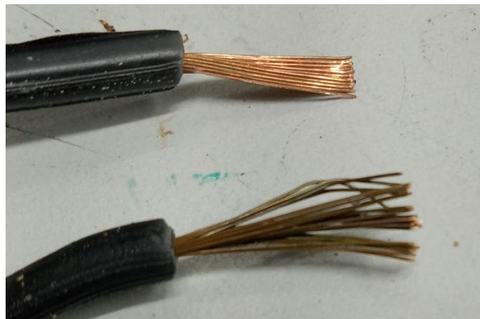
The tarnish (or oxidation) introduces resistance into any connection with the wire reducing the capacity of the connection to carry electricity to the lamps and thus causing the lamp to dim. In an extreme case the oxidation can become so great as to completely block the flow of electricity causing the lamp to turn off.
