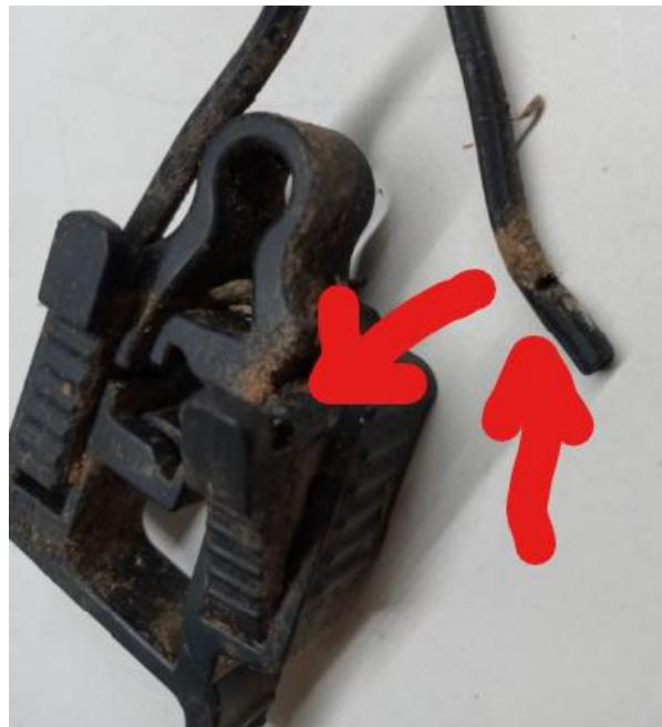
As you can see in the image above this connection is less than ideal and deteriorates over time. Temperature changes, vibration, introduced water freezing, and oxidation all contribute to this connection failure.
