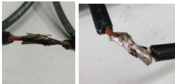
You can see (on the left) that the no flux solder connection is very poor, and that (on the right) the flux connection looks very nice and shiny.
